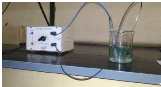
Figure 1: Experimental setup for electrolysis of copper sulphate
