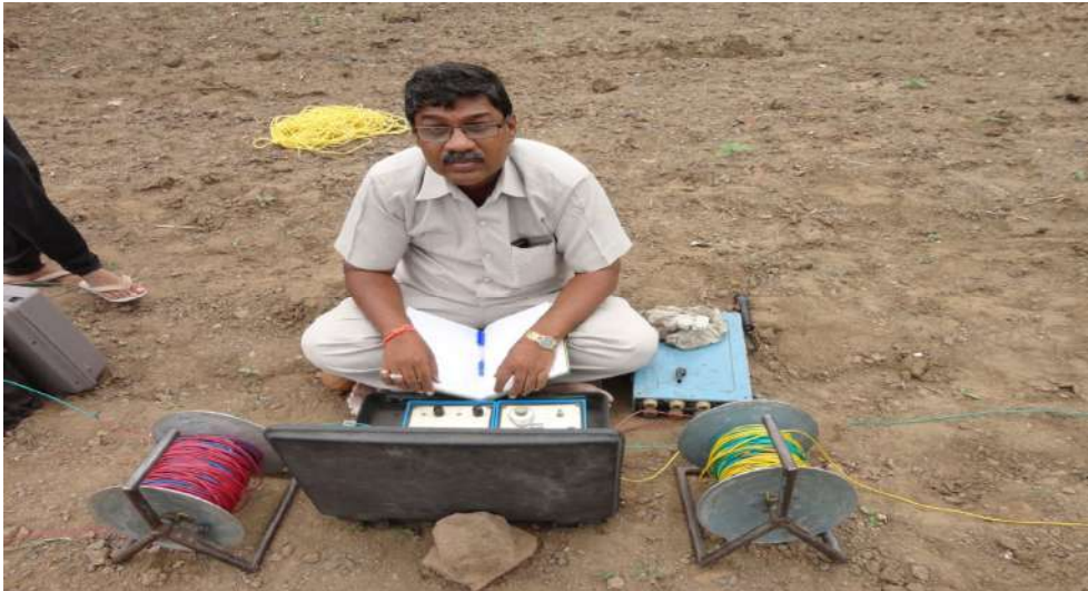
Photo 1 : Shows resistivity survey for subsurface rock identification
