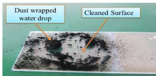
Fig. 3: Self-Cleaning property of superhydrophobic coating.
