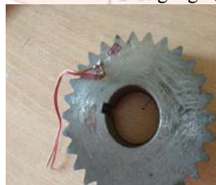
Fig.8. Bonding of strain gauge
